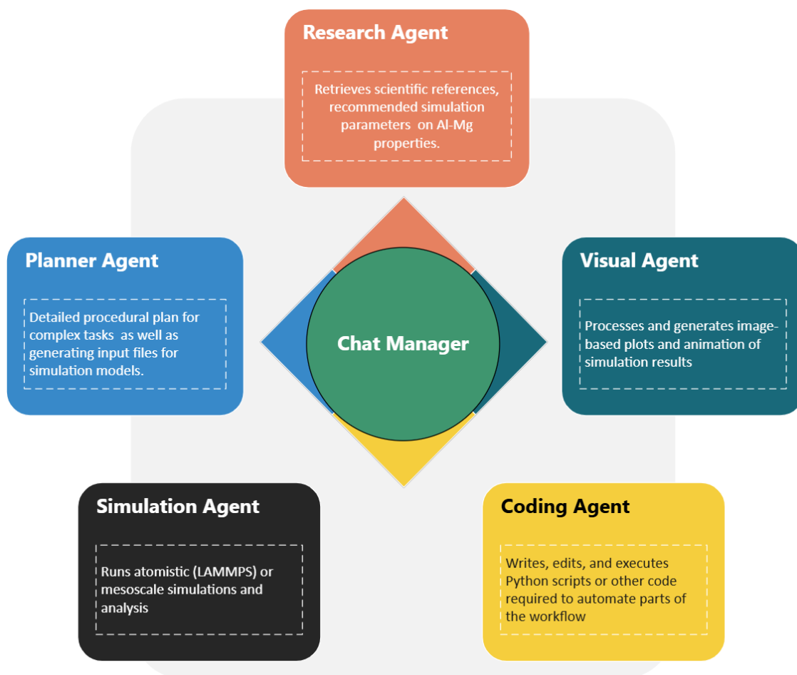
Figure 1. Multi-agent orchestration framework for LAMMPS simulation of Al alloys.
